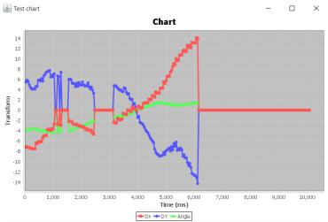
This chart is generated after the transformation is run. This shows the user a graphical representation of the computed transformations (translations in x and y and rotations). After this step the user can use the computed transformations and apply them to a specific channel. So assume he / she computes the transformations on the red channel but wants to apply them to a different channel he can do that in the alignment step shown below in the figure:
