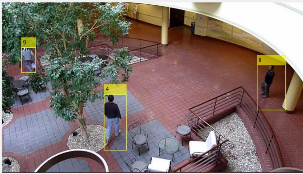
Figure 10: Kalman Filter being used to track multiple objects in a video
